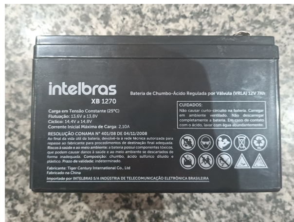
Figure 17 – Pioneer 2DX - Batteries Informations
