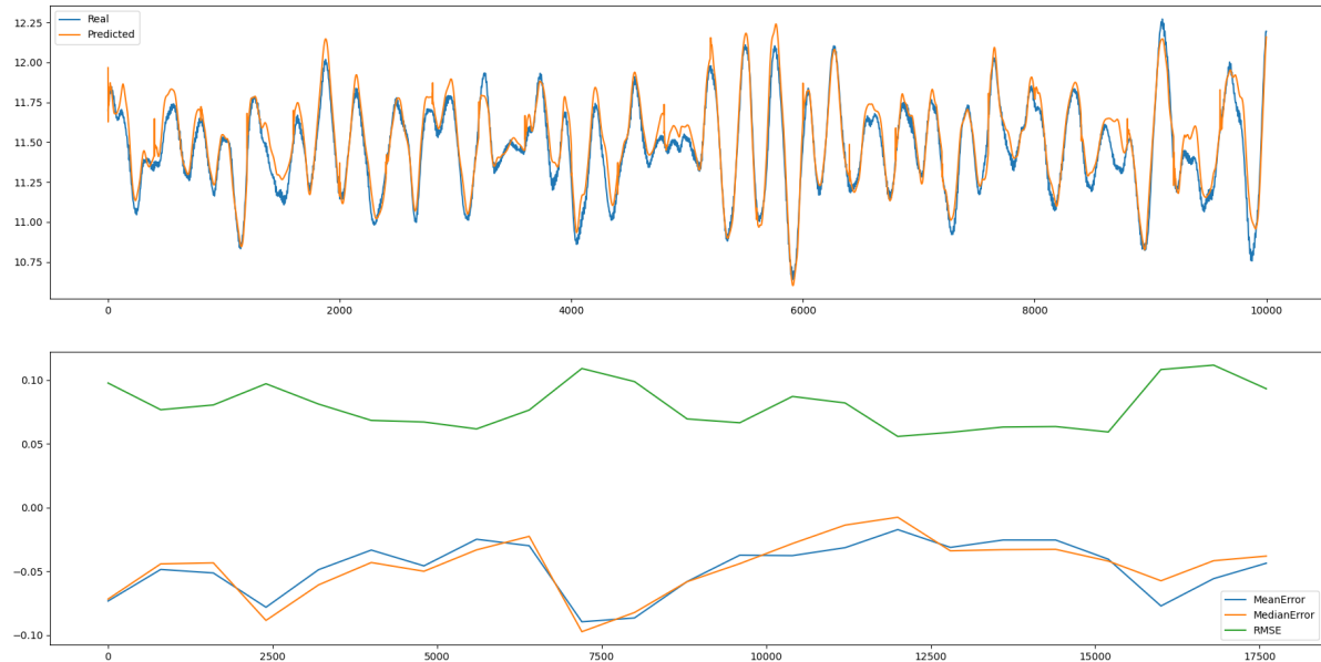
Figure 44: Error Calculation. Top: predicted (orange) and actual (blue) motion values. Bottom: RMSE (green) median (orange) and mean (blue) error scores for each error window.
